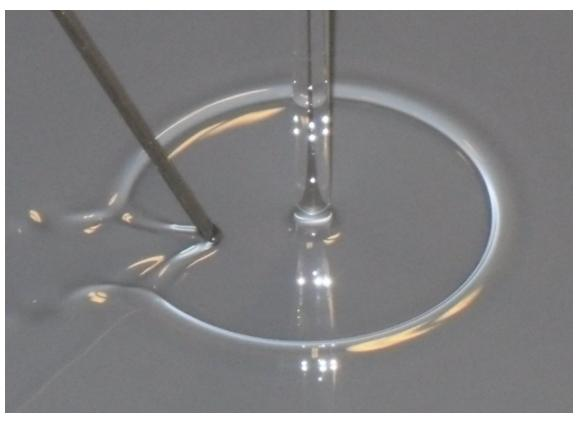
Hydraulic jump around a fluid jet falling on a flat surface. From the work of G. Jannes, R. Piquet, P. Maïssa, C. Mathis, and G. Rousseaux Phys. Rev. E 83, 056312
